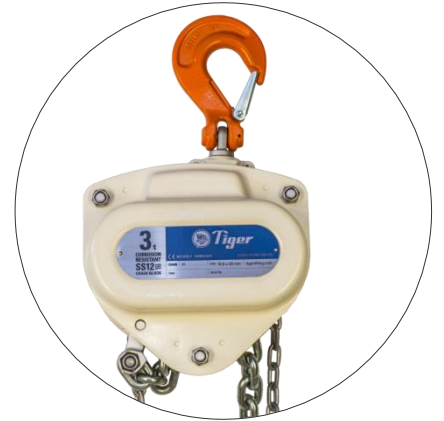
SS12 chain block with clevis adaptor and self-locking (safety) hook, reeveable egg (master) link and sling hook fittings
