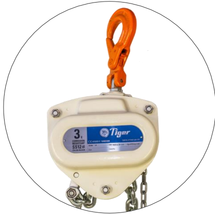
SS12 chain block with clevis adaptor and self-locking (safety) hook, reeveable egg (master) link and sling hook fittings
