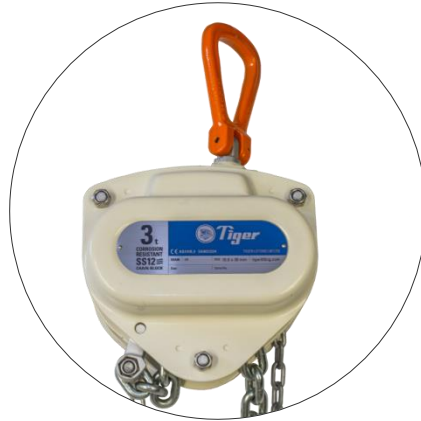
SS12 chain block with clevis adaptor and self-locking (safety) hook, reeveable egg (master) link and sling hook fittings
